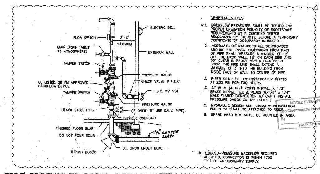
FIRE SPRINKLER RISER DETAIL WITH WALL MOUNT FD CONECTION
